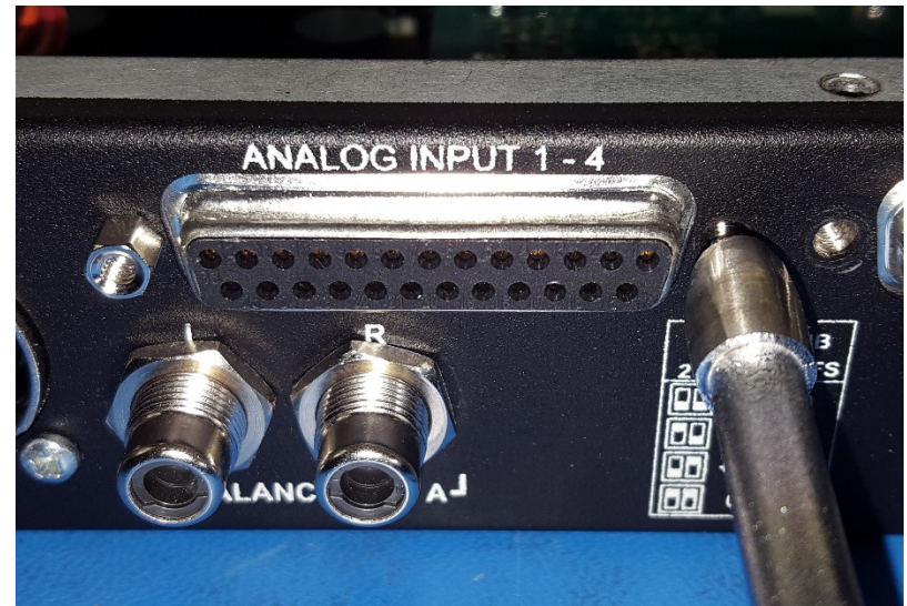
7. Secure option card to rear panel using jackscrews.
